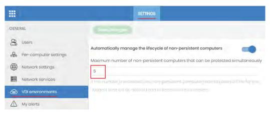
Figure 6.7: Configuring the number of licenses assigned to non-persistent VDI computers
